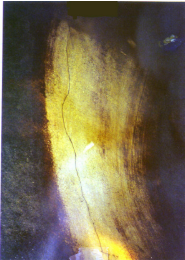
Photo #13: Circumferential crack in 42" P.L. south of Location 1.
